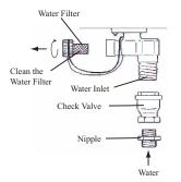
Notice: Use only teflon tape on cold and hot water connections and lines.
